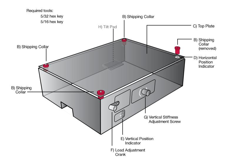
DO NOT REMOVE SHIPPING COLLARS UNTIL INSTRUCTIONS INDICATE. SHIPPING COLLARS MUST BE USED WHEN MOVING ISOLATOR.
