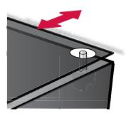
9. The horizontal natural frequency can only be changed by varying the payload weight. Approximately 1.5 Hz is achieved when the payload weight is near the nominal (ie. 25 lb. for the 25BM-10). Increasing the weight lowers the frequency. Decreasing the weight raises the frequency. Ballast weights can be used to adjust the frequency.
