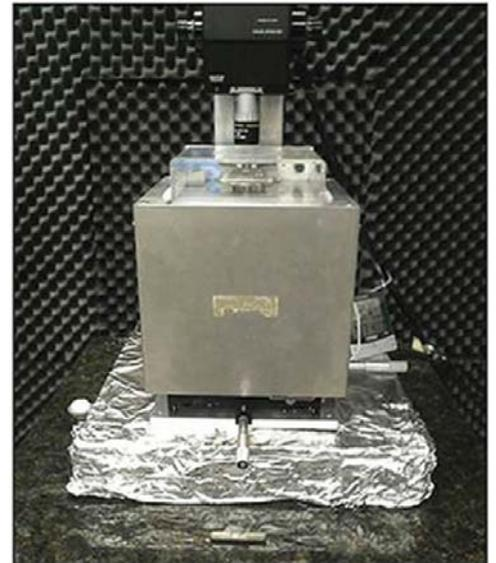
*SLU's negative-stiffness vibration isolation system.*
