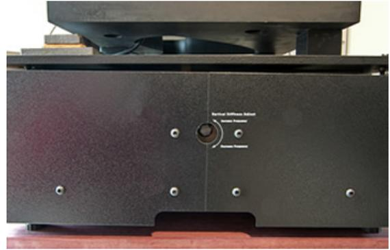
Vertical position indicator and the crank below it for that adjustment.
