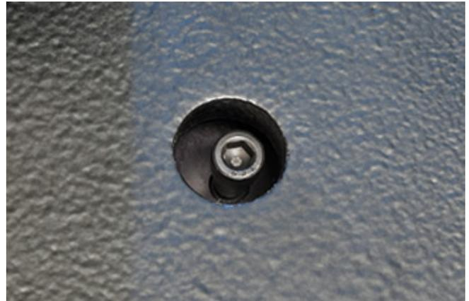
With the transit plugs removed, the allen bolts are threaded back into the fixture, to serve as a visual guide for loading adjustments.
