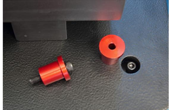
**transit plugs. These fit down into the 4 holes, of which one is seen to the right, and use the allen bolt to thread into the fixture beneath. With the four transit plugs installed the suspension system is immobilized for safe shipping and storage. These have to be removed at installation but come in handy when loading and unloading the platform because they --- immobilize-- the suspension during setup procedures.**
