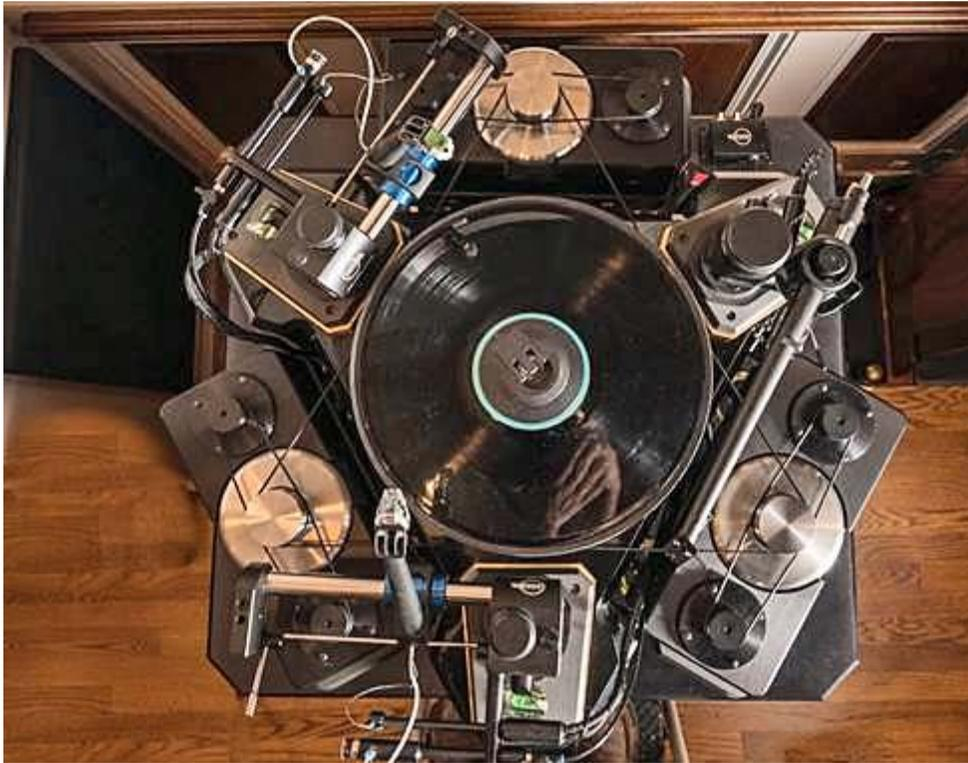
*The turntable's 3 drive pods, each with 2 synchronous motors, drive a 15 lb. flywheel.*
