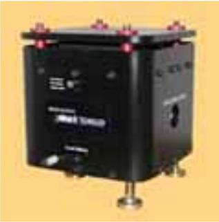
Minus K Technology has released a compact, high-capacity, low-frequency negative-stiffness isolator designed to support heavy payloads while reducing low-frequency vibrations. The new CM-1 isolator comes in several capacity ranges to match vibration-sensitive instruments such as SPMs (AFMS, STMs, etc), micro-hardness testers, profilers, interferometers, electron microscopes, or other imaging systems, for weight loads from 50 to 800 lbs.
