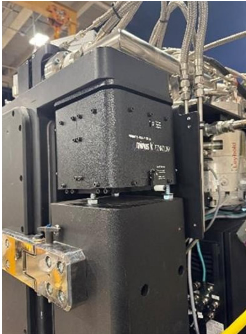
One of the Minus K vibration isolators installed on The Big Fridge. (Image courtesy Maybell Quantum Industries)
