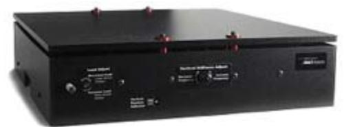
Vibration transmissibility with Negative-Stiffness is substantially improved over air systems, which can make vibration isolation problems worse since they have a resonant frequency that can match that of floor vibrations. Transmissibility is a measure of the vibrations that transmit through the isolator relative to the input vibrations.
