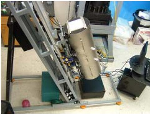
At the SMART Laboratory, crystals of CdZnTe and the scintillator materials are grown via a vertical Bridgman furnace. In this process, molten material is directionally solidified from one end to the other to produce a large-volume ingot that is a single crystal. Methods to grow CdZnTe for gamma-ray spectrometers have been explored since the early 1990s, yet a reliable system to produce large crystals at an economical cost has not been achieved until relatively recently.
