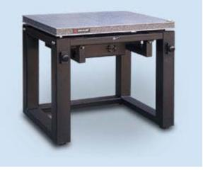
passive isolator capable of very low vertical and horizontal natural frequencies and very high internal structural frequencies, according to the company. Minus K claims its isolators (adjusted to 1/2 Hz) achieve 93% isolation efficiency at 2 Hz; 99% at 5 Hz; and 99.7% at 10 Hz.
