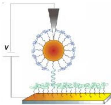
“Schematic of the measuring system – DNA oligomer is attached to a gold electrode below, and hybridizes with a DNA attached to a gold nanoparticle which then forms the upper electrode for the double-stranded DNA. Current is measured by applying a bias between upper and lower electrodes with placement controlled by the AFM tip – Weizmann Institute.”
