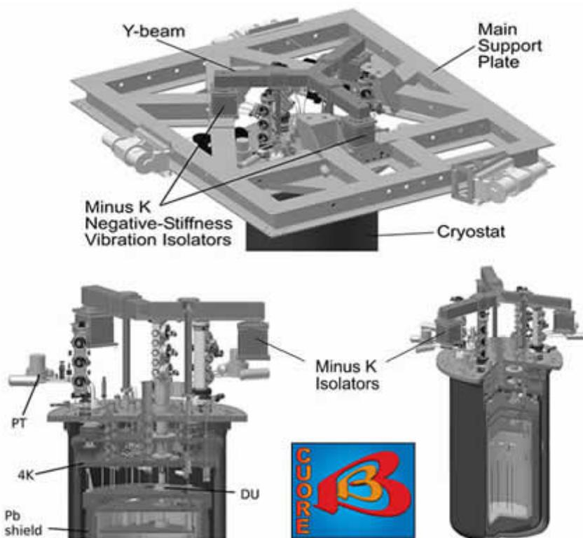
Italy's National Institute of Nuclear Physics (INFN) has installed three custom vibration isolators for experiments within the Cryogenic Underground Observatory for Rare Events (CUORE), located within Gran Sasso mountain, the highest peak in the Apennines about 100 km (62 miles) from Rome.
