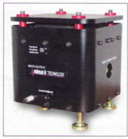
Horizontal natural frequency is load dependent, with ½ Hz or less being achievable at or near the nominal load. Completely passive, the isolator uses no air or electricity. It can be made cleanroom and vacuum compatible, and several units can be combined into a multiisolator system to support heavy payloads.
