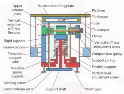
The negative-stiffness vibration-isolation system uses three subsystems to isolate the payload from vibrations. The support spring, combined with the vertical negative-stiffness flexures, clamp, compression spring, and vertical-load and stiffness-adjustment screws, isolates the system from vertical vibrations. The beam-columns perform horizontal isolation. And the tilt flexure and damper isolate tilt vibrations from the payload.
