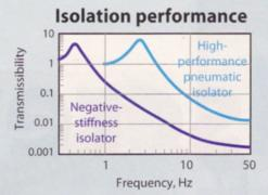
Negative-stiffness isolators have resonant frequencies at 0.4 to 0.5 Hz, compared to 2.3 Hz for pneumatic systems. They transmit less energy from low-frequency vibrations to the payload than do pneumatic systems, and maintain better isolation performance through building frequencies to about 100 Hz.
