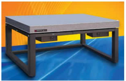
The MK52 negative-stiffness optical vibration isolation table achieves vertical and horizontal natural frequencies of 0.5 Hz or lower without limiting its ability to support static loads. At a natural frequency of 0.5 Hz, it provides isolation efficiencies of 93% at 2 Hz, 99% at 5 Hz, and 99.7% at 10 Hz.
