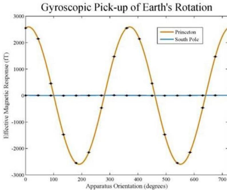
*Comparison of the gyroscopic pick-up of the Earth's rotation measured in Princeton and at the South Pole.*
