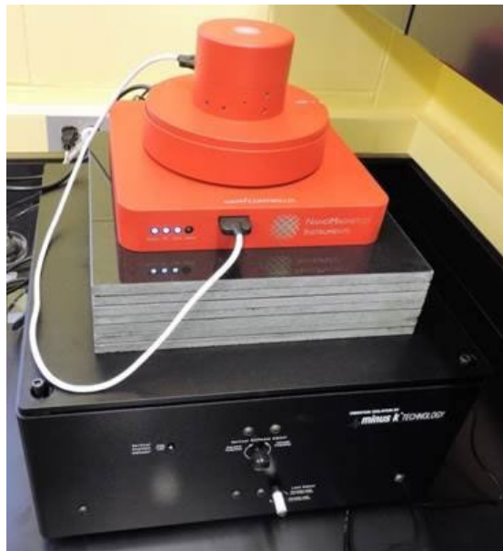
ezAFM+ supported by Negative-Stiffness vibration isolation.
