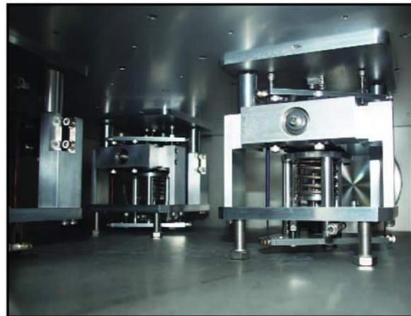
Minus K Negative-Stiffness vibration isolators inside the GEO600 vacuum chamber
