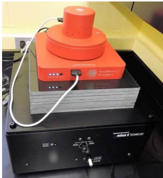
ezAFM+ supported by Negative-Stiffness vibration isolation.
