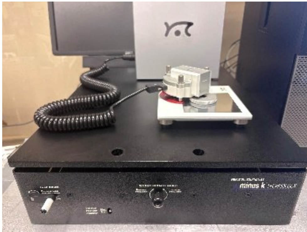
AFM positioned on top of the Minus K Negative-Stiffness isolator at the Nanomaterials Lab at the University of North Texas. (Image courtesy University of North Texas)
