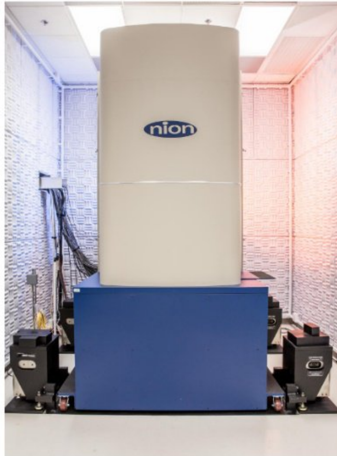
IMRI's Nion UltraSTEM 200 equipped with a high-energy resolution monochromated EELS system and Negative-Stiffness vibration isolation floor platform. (Image courtesy IMRI)
