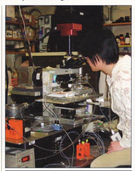
A vibration isolation system that works in both the X-Y and the Z-planes (the Nano-K device immediately under the microscope) is allowing researchers to study neuron activity with micron resolution. The system acts as the negative of a spring and thus drastically reduces ambient vibrations with especially low natural frequencies.
