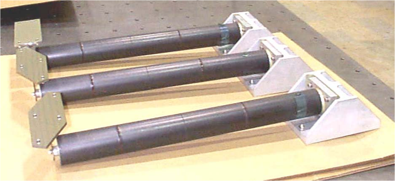
Figure 4. Backpack Isolator Struts Prior to Installation
