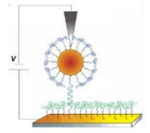
"Schematic of the measuring system – DNA oligomer is attached to a gold electrode below, and hybridizes with a DNA attached to a gold nanoparticle which then forms the upper electrode for the double-stranded DNA. Current is measured by applying a bias between upper and lower electrodes with placement controlled by the AFM tip – Weizmann Institute."
