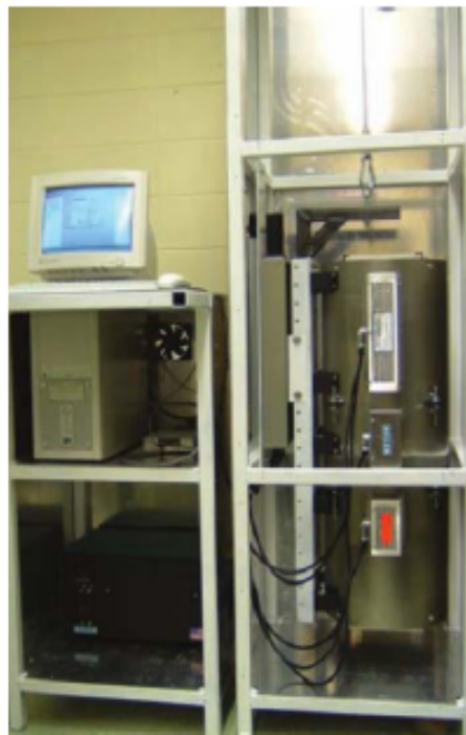
Left: Conventional vertical Bridgman furnace used to grow the semiconductor material, cadmium zinc telluride (CdZnTe).
